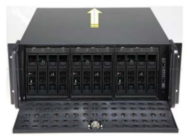
1. Remove the screws from each side of the Chassis. (two on each side)
